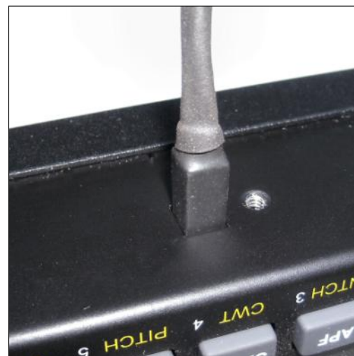
The plug allows two keys to be used with the KX3.
