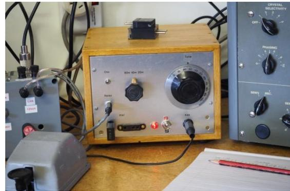
The chassis and front panel are aluminium, folded on a home brew bending brake. Where once a chassis punch would have been used to make valve socket holes etc. (expensive!) I now use a step drill which works well in aluminium. The case is made of solid English oak which again came from recycled old bed ends and then finished with Shellac.
